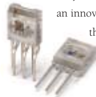
Tiny devices like these send and receive light signals via plastic fiber.
